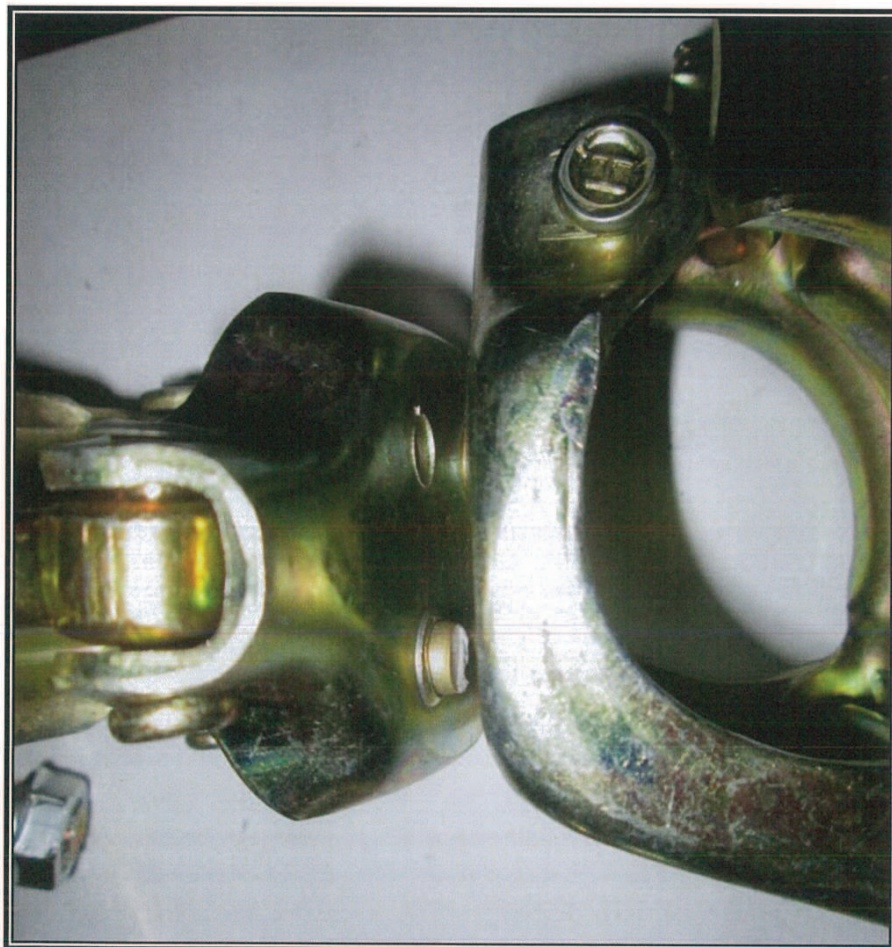
Photograph 6: Shows failure mode of the tested sample - Set 2
