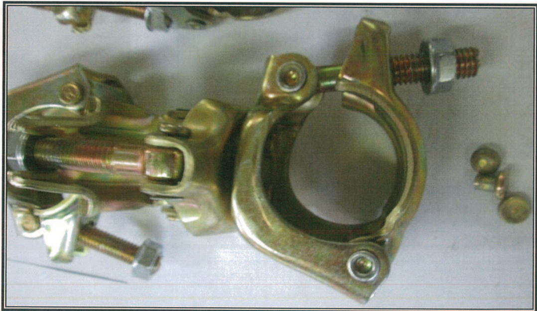
Photograph 4: Shows failure mode of the tested sample - Set 1
