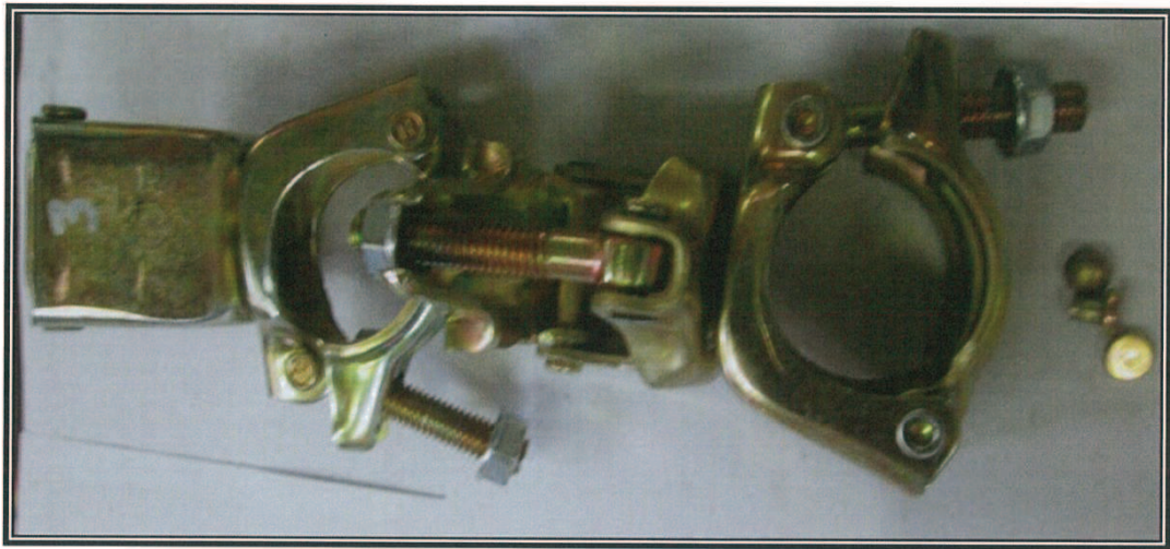
Photograph 7: Shows failure mode of the tested sample - Set 3
