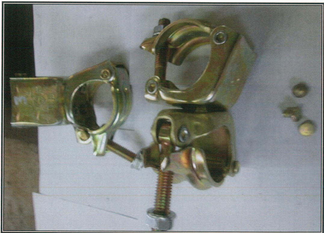
Photograph 8: Shows failure mode of the tested sample - Set 3
